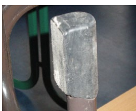
Sharp-edged, damaged, worn and unsuitable, soiled chair glides
