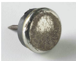
Metal slides with adhering dirt after seven months of use
