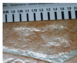
Lasting indentations due to high point load and hard glides
