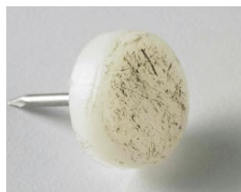
Highly damaged nylon glides after three to four months of use
