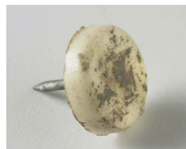
Nylon glides with thick dirt adhesion after eight months of use
