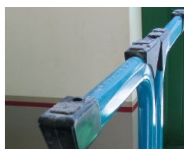
Sharp-edged, damaged, worn and unsuitable, soiled chair glides
