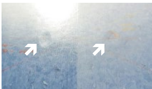
Fig. 5: Visibility of the indentations after loading depending on the level of gloss [1]
