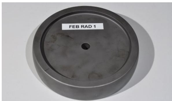
Fig. 3: Test wheel made of steel (reference wheel) [2]
