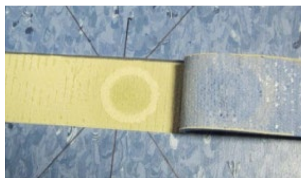
Fig. 6: Adhesive compression after loading [1]
